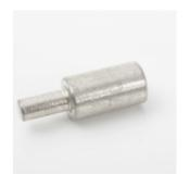
The Termination Technology range of bare Solid Reducing Pins are designed to reduce down conductor size when cables are oversized for control gear and MCB's. The pin makes these terminals ideal for terminating conductors into contact blocks. The range covers sizes from  $10 \text{mm}^2$  to  $400 \text{mm}^2$  with larger sizes up to  $1000 \text{mm}^2$  being custom made to request.
