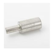
The Termination Technology range of bare Solid Reducing Pins are designed to reduce down conductor size when cables are oversized for control gear and MCB's. The pin makes these terminals ideal for terminating conductors into contact blocks. The range covers sizes from 10mm<sup>2</sup> to 400mm<sup>2</sup> with larger sizes up to 1000mm<sup>2</sup> being custom made to request.
